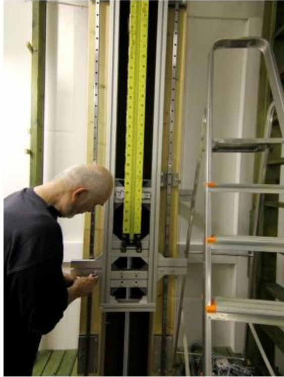
Leveling comparator constructed by FGI
