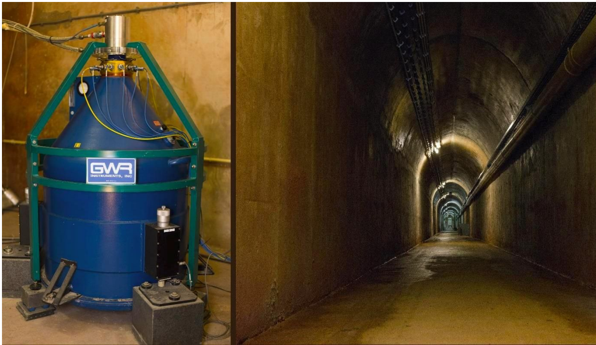
The superconducting gravimeter is located at the end of a 132 m – long gallery, 48 meters underneath the surface, in Membach (city of Baelen, eastern Belgium). The instrument sensor is immersed in liquid helium in which the temperature is held at -269^{\circ}\text{C} , in other words 4 degrees above absolute zero, allowing superconductivity. Photo credits: E. Coveliers (gravimeter & gallery); B. Frederick (Sensor)
