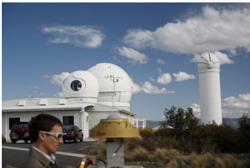
Figure 1.4: Mount Stromlo fundamental geodetic observatory, with GNSS in foreground of image, and SLR station centre of image
