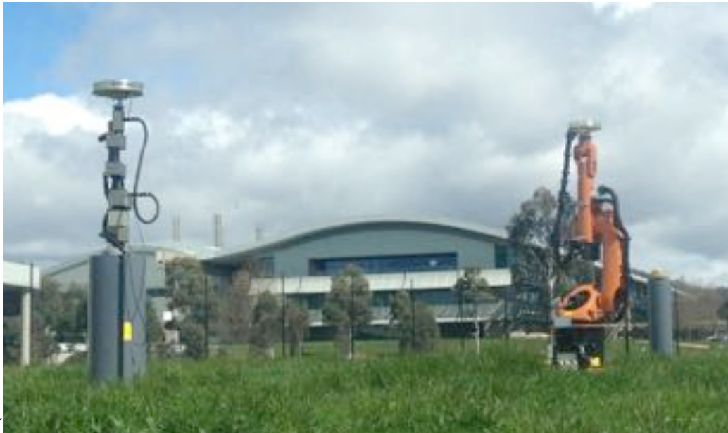
Figure 1.7: The Geoscience Australia antenna calibration facility, Canberra
