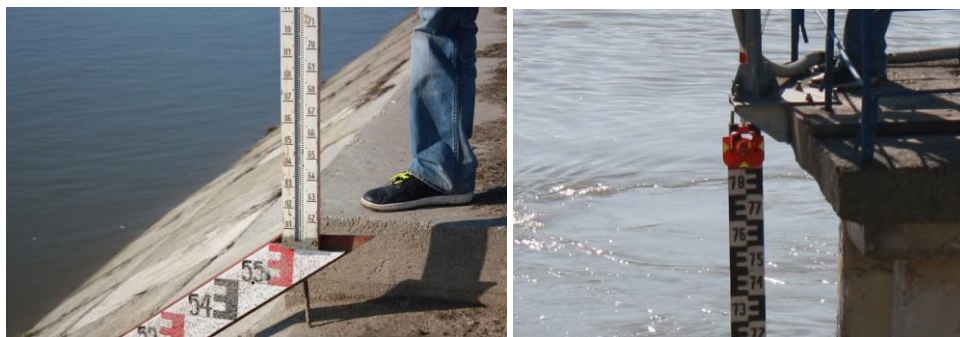
Figure 9. Height determination for the depth gauges (geometric / trigon. levelling)
